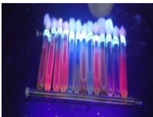
Fig. 3: The fluorescence analysis was observed under long UV (365nm).
